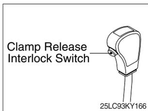
(1) When the lever is operated on pressing this clamp release switch, the clamp opening or releasing function is activated.
