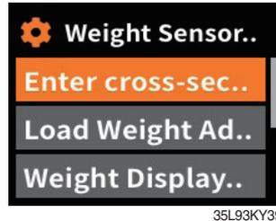
Choose Cylinder Cross-Section. If Cylinder Cross-Section is already set up, setting value is shown in initial screen.
